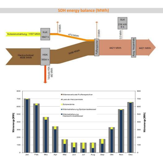
For the reference case the solar fraction obtained is of 6.3% with flat -plate collectors, 10.4% with CPC collectors\*.
