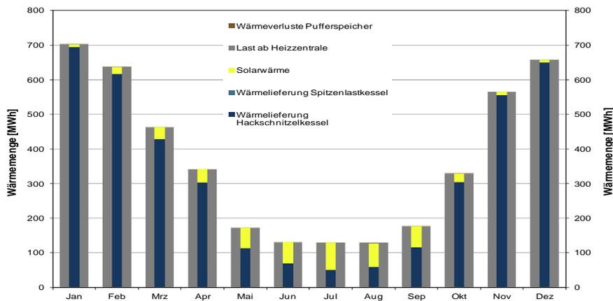
For the reference case the solar fraction obtained is of 6.3% with flat -plate collectors, 10.4% with CPC collectors\*.
