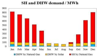
Finally whole district heating energy balance is presented including influence in production and distribution loses, with and without solar installation:
