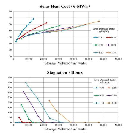
From figures was decided that system configuration combining collectors total area of  $6.595,15m^2$  (Area-Demand ratio of 0,9 m<sup>2</sup>/MWh; purple line) and storage volume of 19.785,56 m<sup>3</sup> (Volume-Area ratio of 3,0 m<sup>3</sup>/m<sup>2</sup>) looks promising for a solar fraction of 60,12% and solar heat cost of 57,47  $\in$ /MWh. Besides, no stagnation hours are considered with this configuration.
