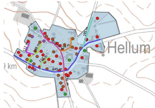
Step 2: Estimation of heat demand in case area (based on building category and age) in a GIS, basic design of DH-grid.
