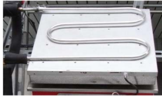
Small meander tubing on heating plate
