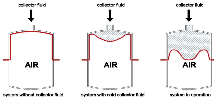
Figure 8.1.3. Cross section of expansion vessel in different situations. (Source: CityPlan – based on [4])
