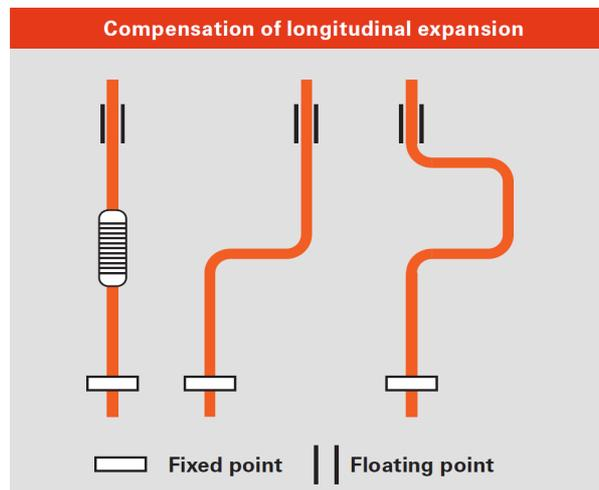
Figure 8.1.2. Pipes including compensation for longitudinal expansion [3].
