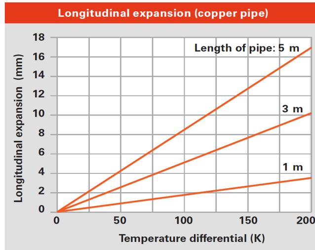
Figure 8.1.1. Longitudinal expansion of copper pipes [3]. As seen in table 8.1.1 the expansion is almost 30 % larger than for steel pipes.
