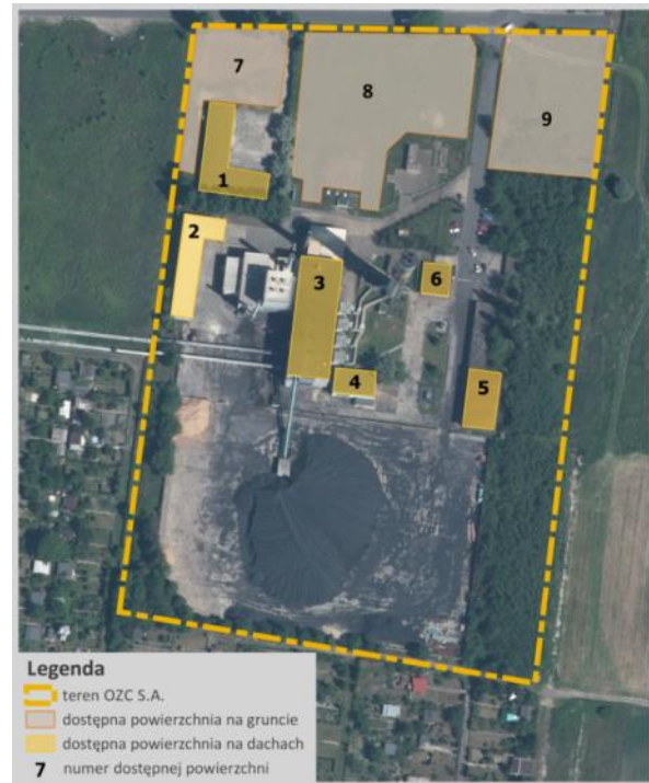
Figure 2 The area available on the heat and power plant, source: IEO
